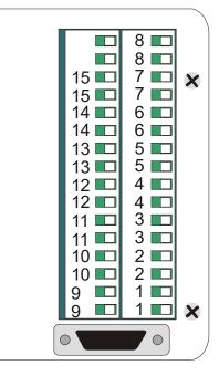
Wiring of thermo resistors (Pt100 3wire) for CR15+
