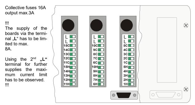
The 3 output-boards are electrically isolated from each other as well as from the unit itself. That is why the 3 boards have to get supplied separately. For 3-phase installation the 3 boards may be used for the 3 phases(L1, L2, L3).
