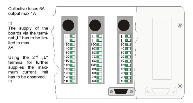
Definition of the terminals for low-voltage outputs (24 V DC)
