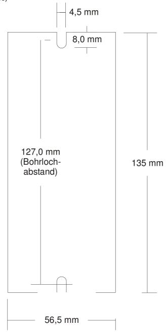
The FP08 is designed to get fixed to the mounting plate by 2 screws M4.
