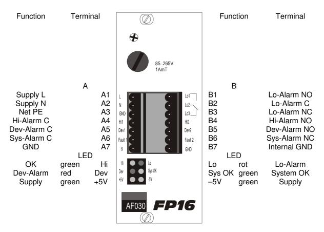
The supply is accepted from 85VAC to 265 VAC. Frequency 50/60 cps Fuse 1,0 A mT
