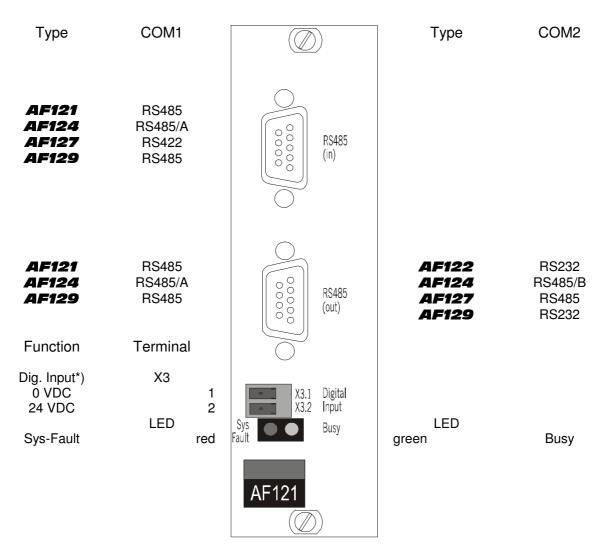
The interface COM1 is available at both plugs, it is linked internal. \*) Function according to parameter settings
