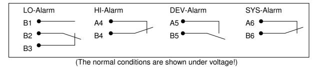
The contacts are potential free and loadable up to 2 amps at 250volts.
