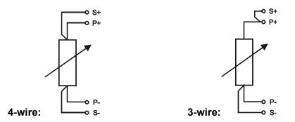
The measurement inputs S+ and S- must be connected or bridged.
